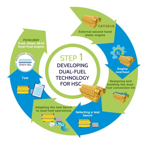
In order to develop the dual-fuel technology required for HSC, a second-hand sister engine with the same characteristics as the four main engines on board the vessel was bought by Fred. Olsen, as the CAT3618 engines were discontinued and there are no engines in the market with similar power, weight and volume.
