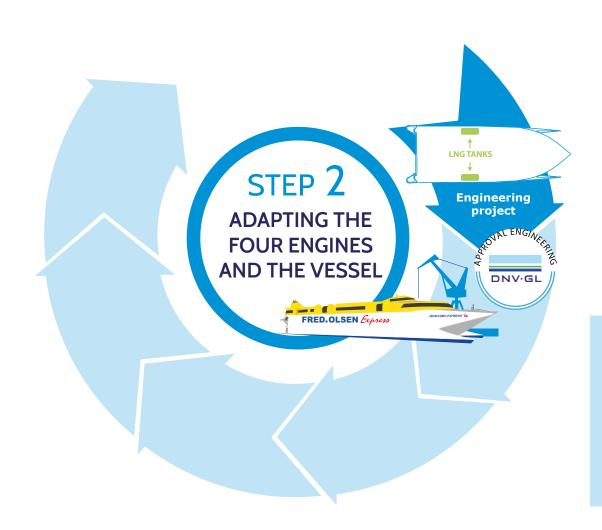
The pioneer technology developed for the adaptation of the propulsion engine to dual fuel will be used to convert the four CAT3618 engines currently on the Bencomo Express, without any need to replace them with new ones.
