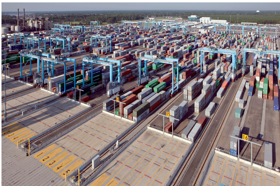
Figura 20. RMGs automáticos (ASCs). APM Terminals Virginia (Port of Virginia – EE.UU.)
