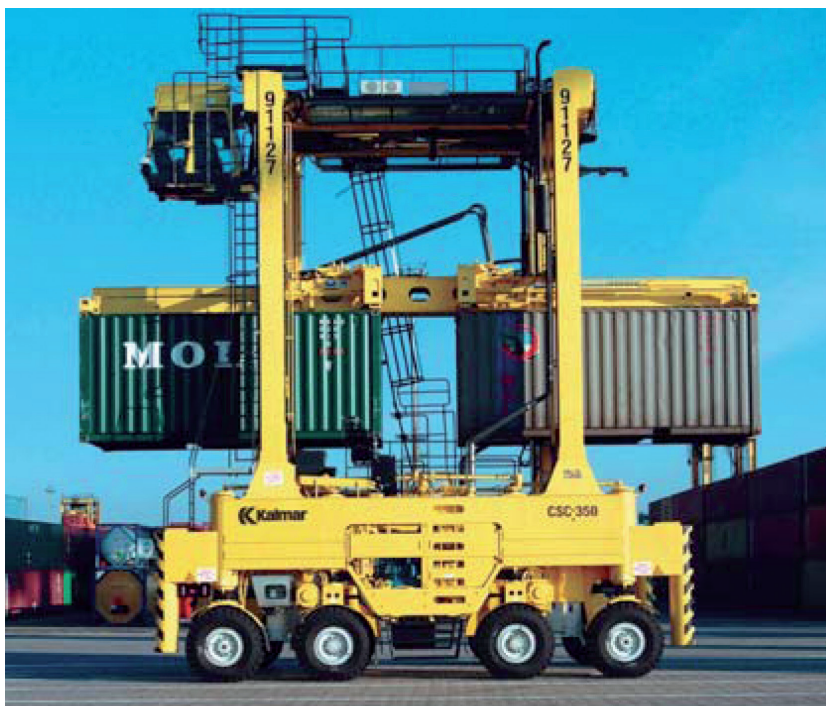
Figura 105. Straddle carrier con spreader twin-lift extensible
