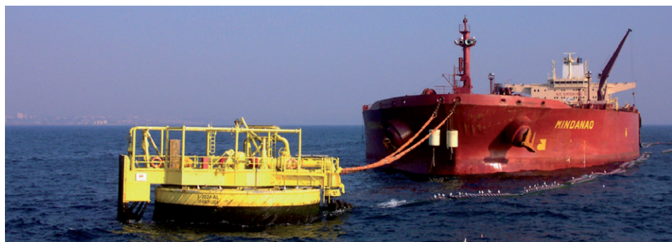
Figure 9. Offshore terminal with single buoy mooring
