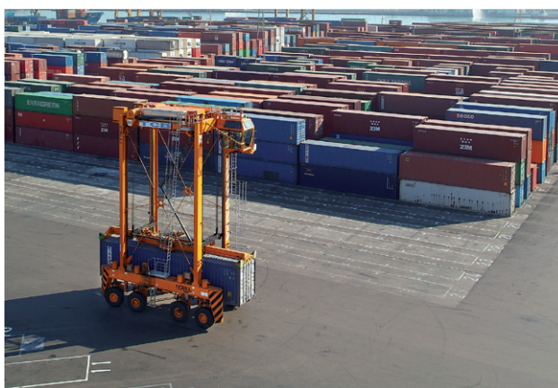
Figure 28. Straddle carrier and storage yard
